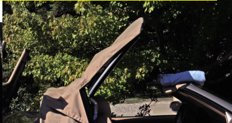
Top position for wave washer and top pin removal
