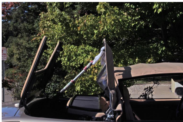
Position for bow cylinder bottom pin, e-clips(2) and pin removal/installation, switch removal/install and main top pin removal/install. Top raised but not latched in front, bow up. Rolled towels to cushion and prevent top from latching in front.
