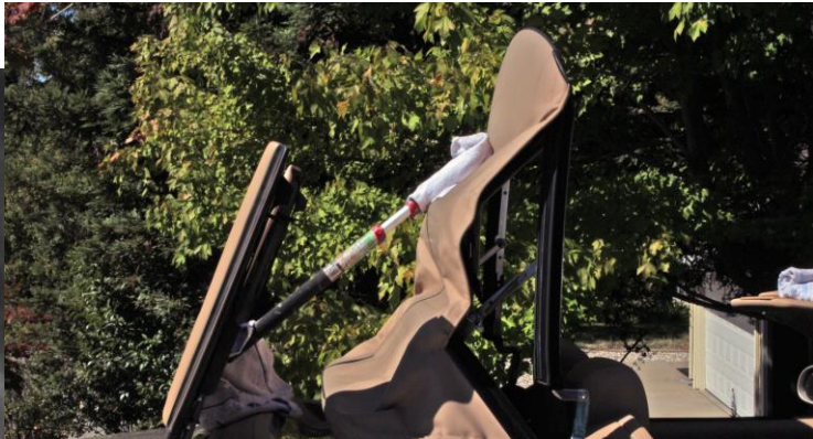
Top position for e-clip and wire guide removal.
